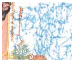
The results of porometric test and blue ink test after NBS crumpling test under different test conditions
