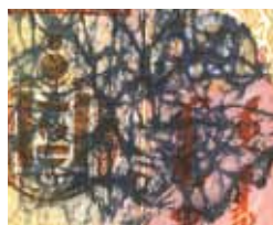
The results of porometric test and blue ink test after NBS crumpling test under different test conditions
