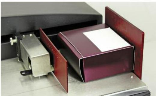
This test ensures that carton based packages can be stacked and displayed correctly. Cartons must also be properly closed to ensure that any secondary process such as film wrapping can be performed.
