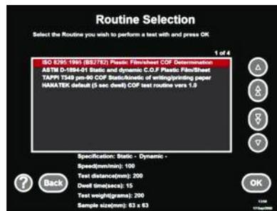
The instrument has pre-loaded test instructions that help ensure samples are tested to international standards
