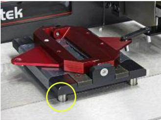
Sled is positioned on lift pins
