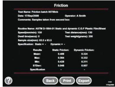
The instrument calculates detailed statistics for multiple measurements. A detailed report can be printed directly from the instrument
