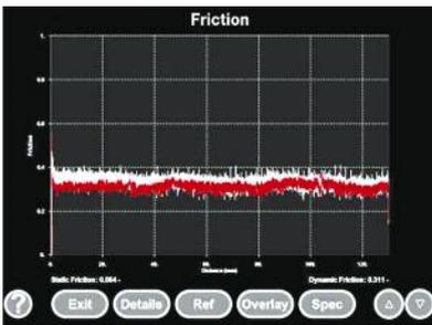
All results can be compared graphically – a previously tested reference can also be overlaid to help understand batch to batch consistency and quality
